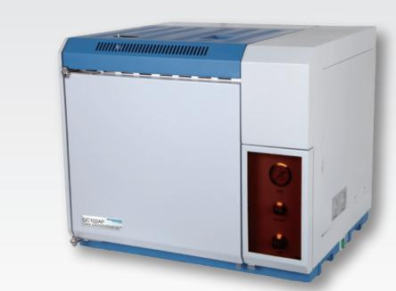
As a new generation instrument, GC102AF Gas Chromatograph applies the computer reverse control technology and canconduct remote detection and fault diagnosis, equipped with a flame ionization detector (FID).
