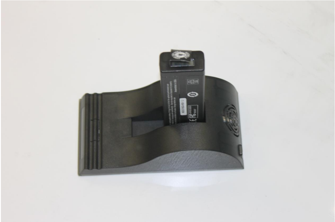
chart : Battery charging interface
