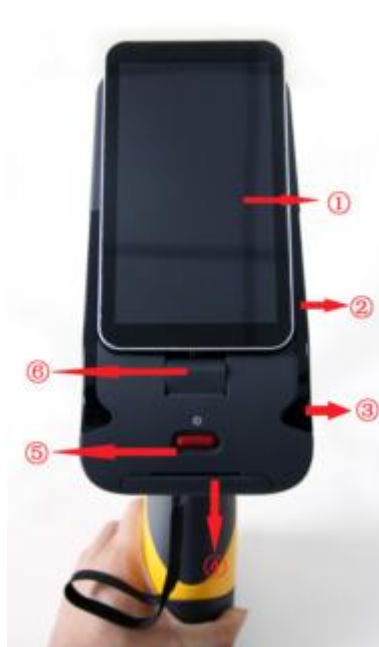
①PDA; ②Radiation Indicator; ③Power Indicator; ④External power port; ⑤ Power switch; ⑥ PDA rotation axis
