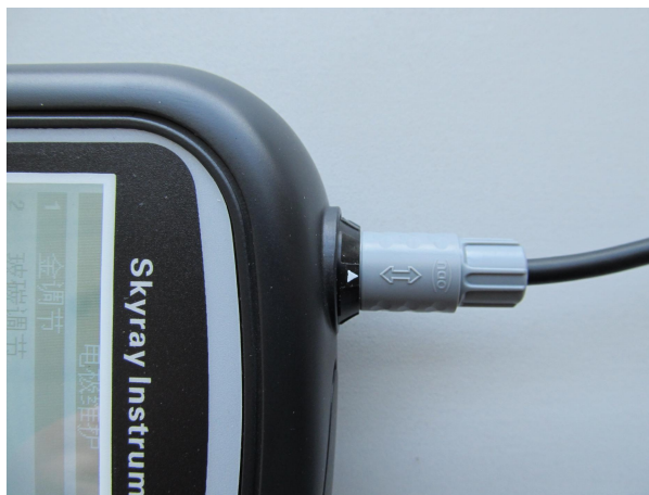
Figure 8 Connection of HM-5000P with electrode device
