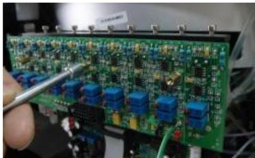
6. Carefully remove the signal process board and put it on the dry and clean place.
