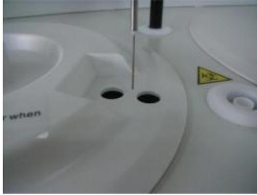
8. Adjust probe position refer to chapter 5.7 sample/reagent probe position adjustment.
