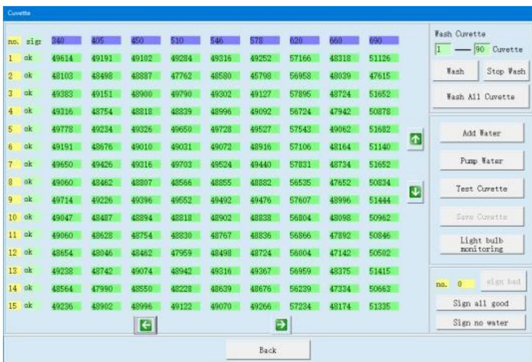
21. Click “Add water” and then click “Test Cuvette” to get the signal value of all cuvettes , observe each wavelength signal value ,it should be between 30000-60000, If the signal value is lower than 30000 or more than 60000, please check related wavelength cuvette. Click “Save Cuvette” and then empty water of cuvettes by click “Pump water” .
