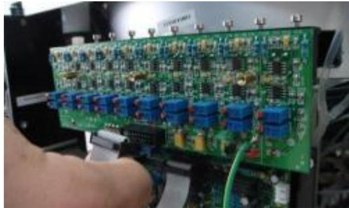
5. Unscrew the three retaining screws of signal process board.
