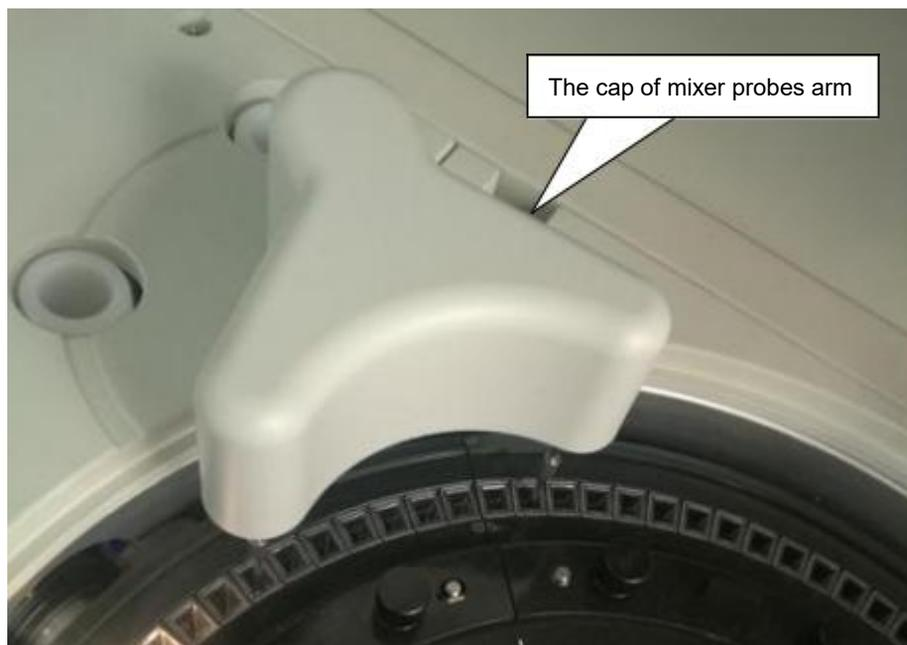
2. Remove the rotary knob of mixer probe and pull out the mixer probe carefully.
