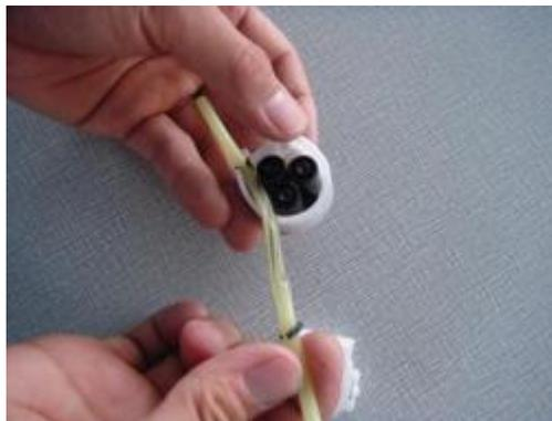
Step 5: If you find the tube was dirty or impressed, you should clean it with gauze and then rub it by hand. and the tube was broken, you can replace.
