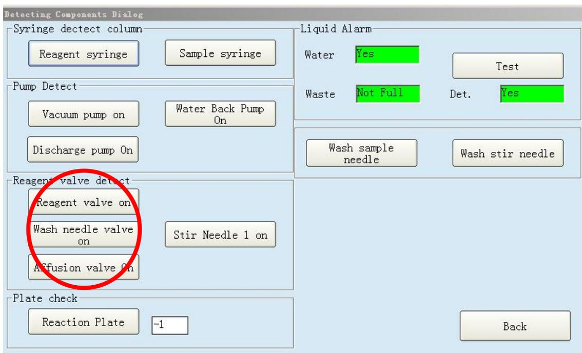
(Respectively click “reagent valve on”, “Wash needle Value on”, “Mix Needle on”, “Affusion valve on”, If the sound “pa” can be heard, then the valves are in good condition; Otherwise, please contact us for help.)
