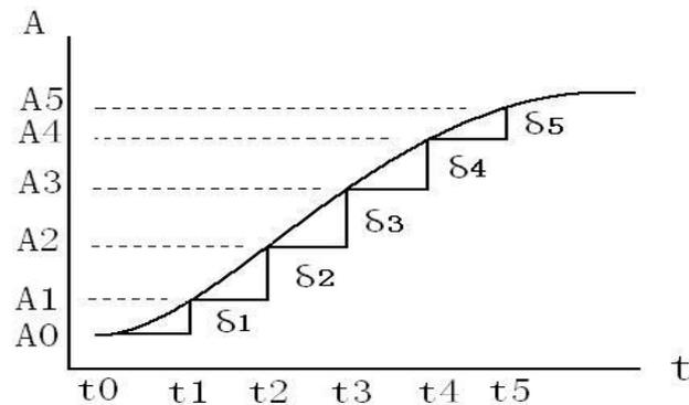
$\delta 1$  and  $\delta 5$  value slants small, and  $\delta 2 = \delta 3 = \delta 4$ , so from A1 point to A4 is linearity section
