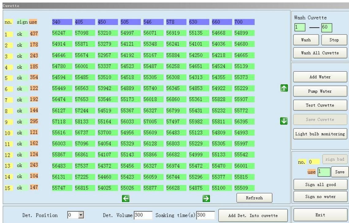
**Note:** please pump cuvettes before testing everyday; and please inject distilled water after test is finished.
