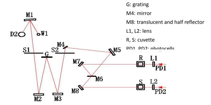
The optical system consists of tungsten lamp (W1), deuterium lamp (D2) and spherical mirror (M1), which reflects the light energy emitted from the tungsten lamp (visible light source) and deuterium lamp (UV light source) and projects it on the incident slit (S1) of the monochromator.
