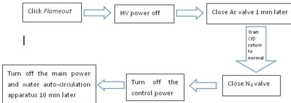
Note: shutdown CID N<sub>2</sub> purge source until CID temp. returns to normal.
