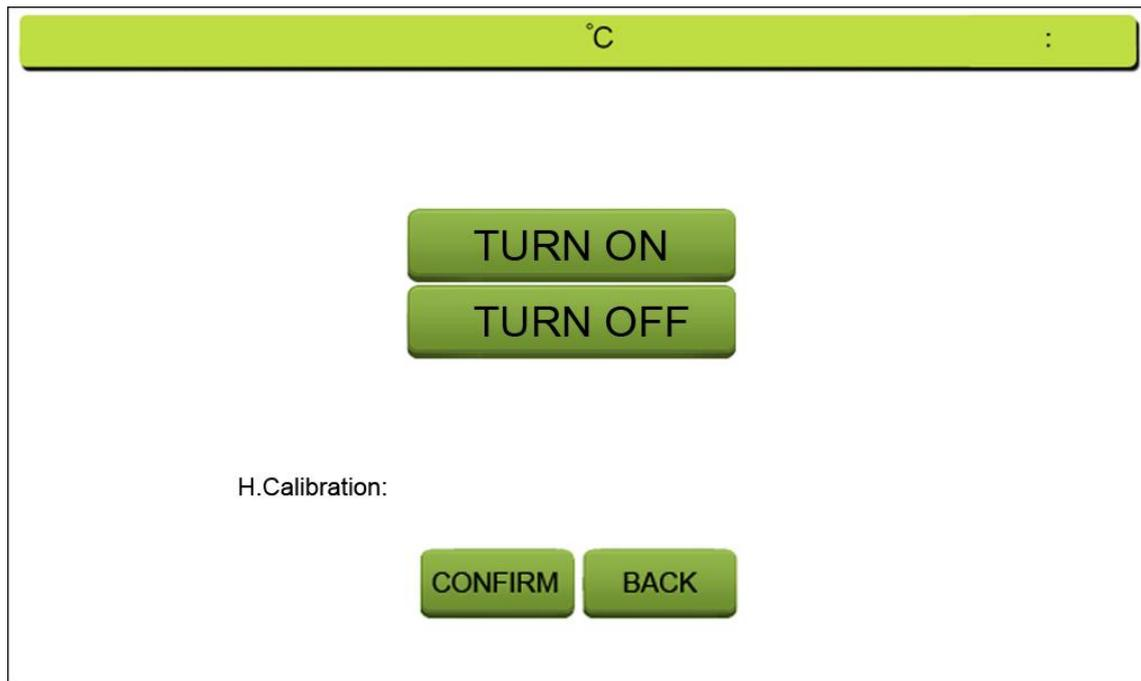
The humidity changed in our environment will effect our moisture test, especially when we test the micro moisture content, it will impact effect the result. So we need turn on this function to keep the result more accuracy.
