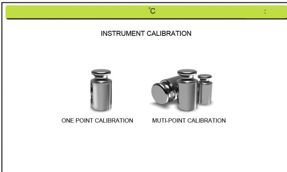
When the instrument error or improper operate . Calibration weights can be adjusted with accuracy. Press "One point calibration" and does not release until it display "-cal-", Then flashing put on the "200.000", put on the calibration weight, then it will display " = = = = =", until it display "200.000", and will show Remove the weight, it will display " = = = = = "again, Waiting it show " 0.000", the calibration is completed.
