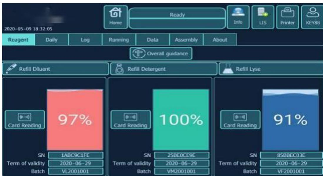
Select the replaced reagent and click "execute reagent guidance" to guide the reagent.
