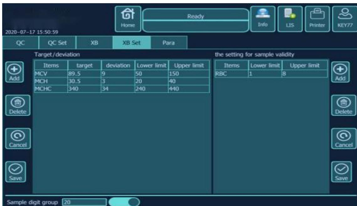
3. In the test items (MCV, MCH, MCHC), set the target value, deviation, upper and lower limit of quality control materials. You can also add or delete other items.
