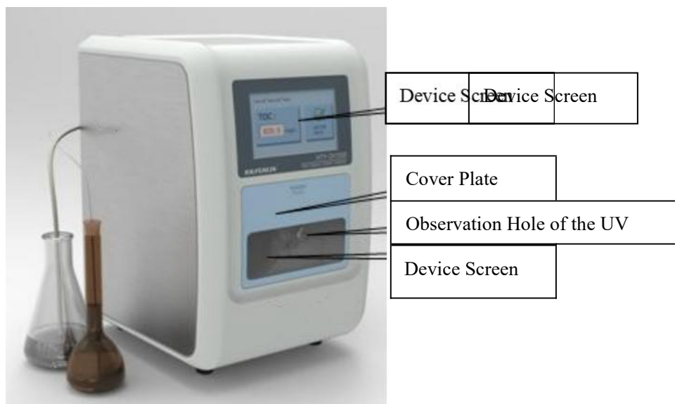
Figure 2-1 Front View of the Device
