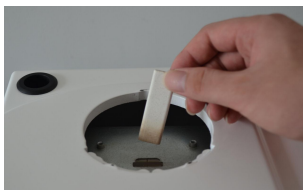
6. Remove the oven core from the broken capillary
