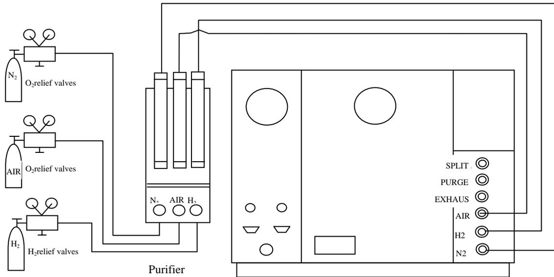
Figure 4-3 Connection Diagram Of Outer Gas Path
