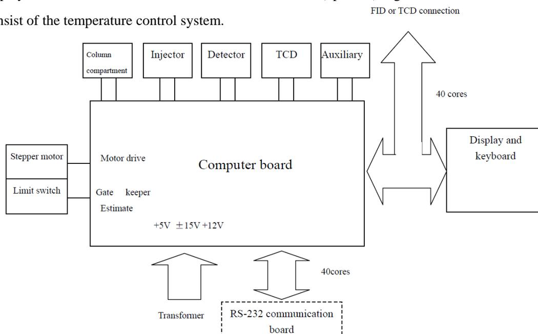
Figure 2-1 Illustration of the microcomputer system
