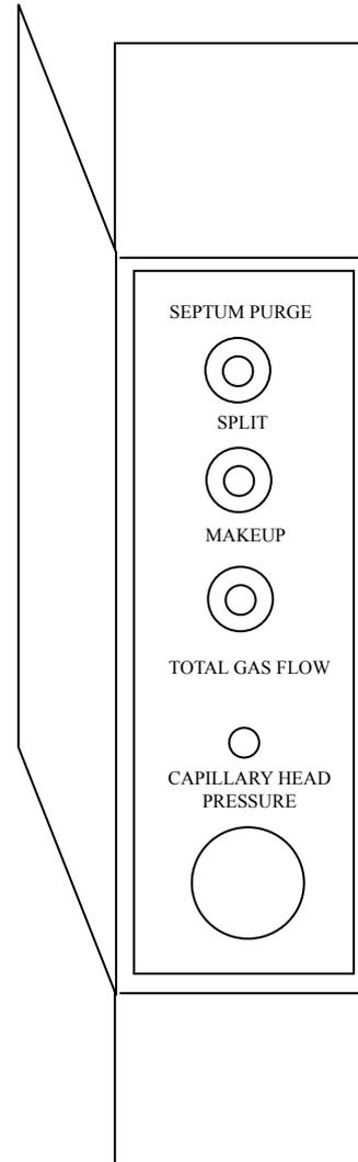
图 1-5 Carrier Gas Regulation Panel (front view)
