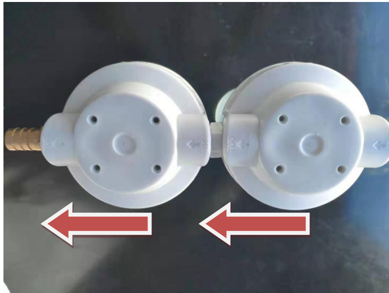
Figure 3-6 Note the direction of the arrow on the cover
