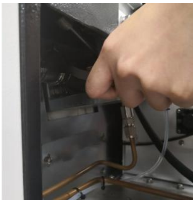
Figure 6-6 Rotating the ball valve
