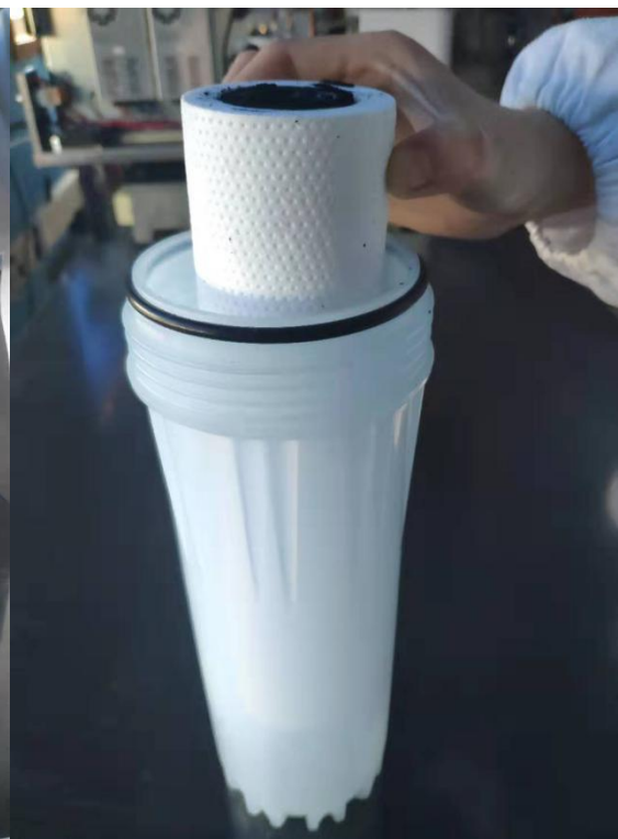
Figure 3-8 Place the filter in the right bottle
