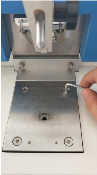
Figure 6-1 Loosening the set screw
