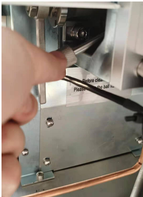
Figure 6-7 Removing the lens Figure
