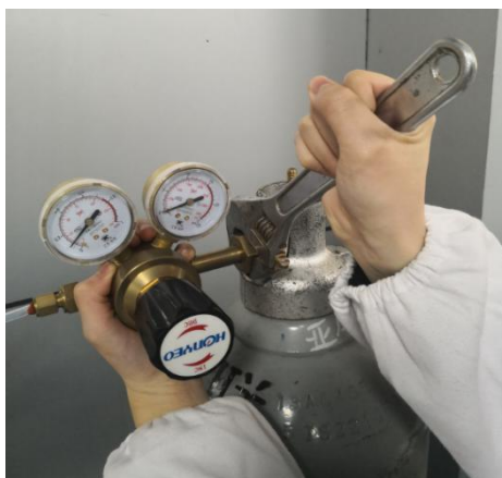
Figure 3-1 The connection between the pressure reducing valve and the argon cylinder should be tightened with a wrench
