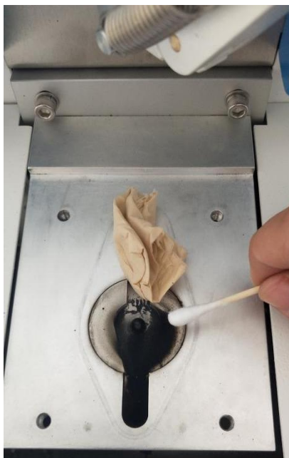
Figure 6-3 Cleaning the spark stand
