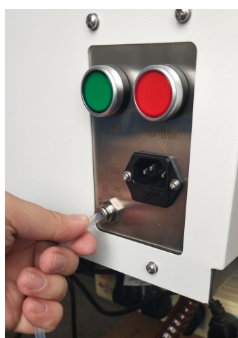
Figure 3-4 Argon inlet behind the machine
