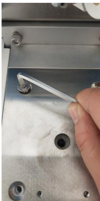
Figure 6-4 Installing the spark stand
