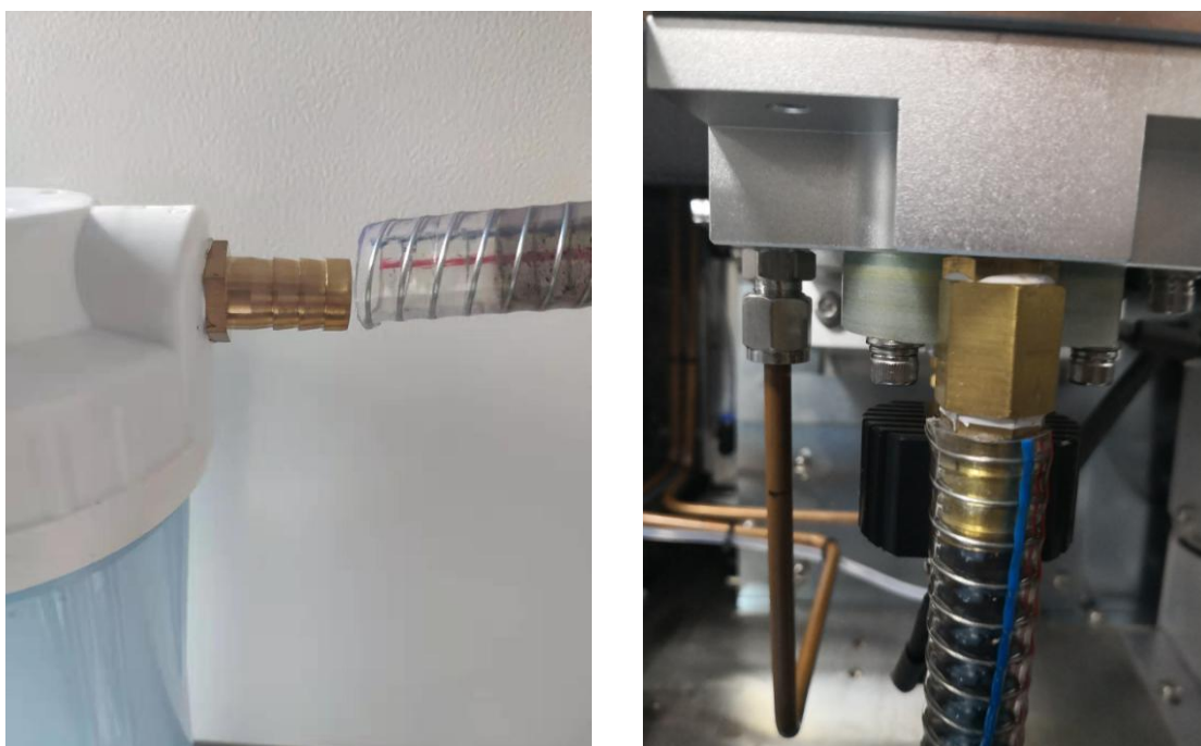
Figure 3-10 Two ends of the gas collection hose
