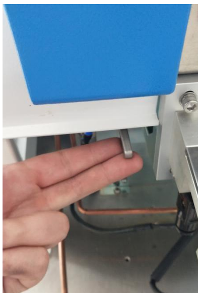
Figure 6-11 Opening the ball valve upwards
