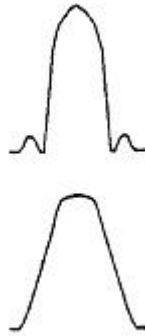
Figure 1-6 A Boxcar Apodized Peak (Top), and the Same Peak After Triangular Apodization
