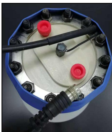
Figure 6-8 Plugs and cable of eluent generation tank
