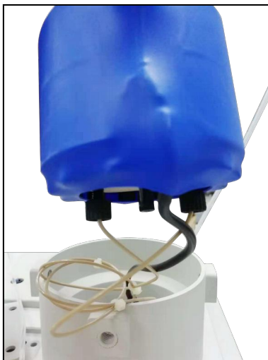
Figure 6-7 Pipeline connection of eluent generation tank
