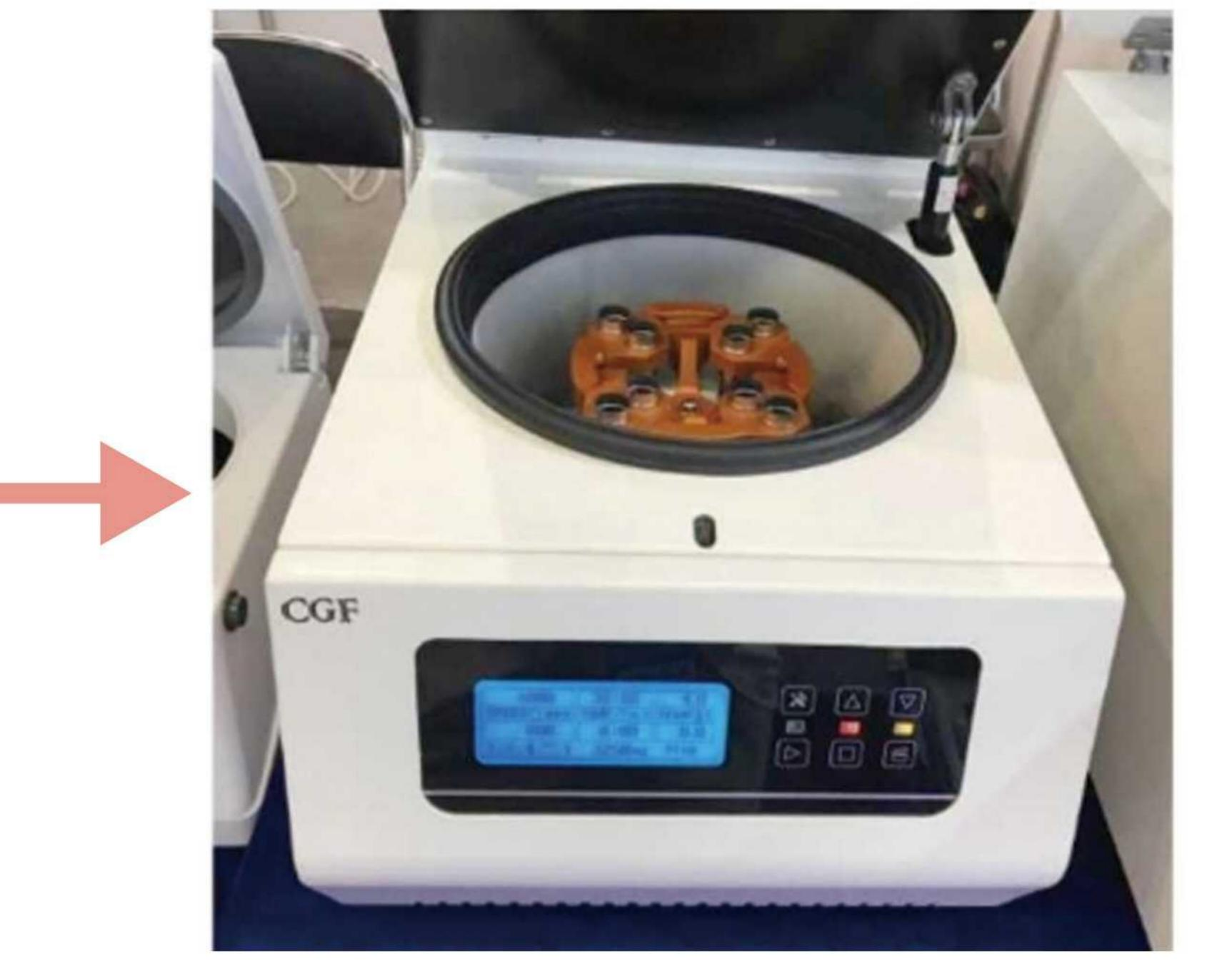
Separate by DL-4M Variable Speed Centrifuge
