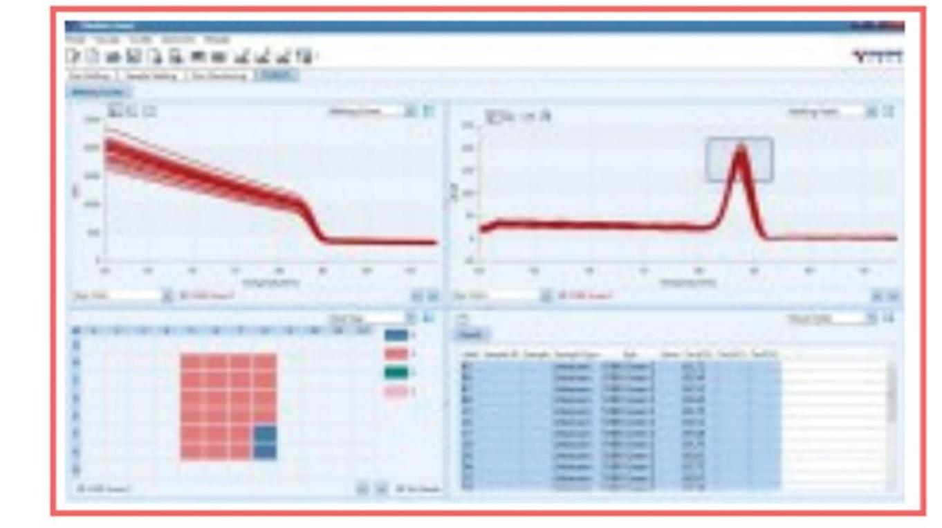
Temperature uniformity of melting curve with SYBR Green I dye.
