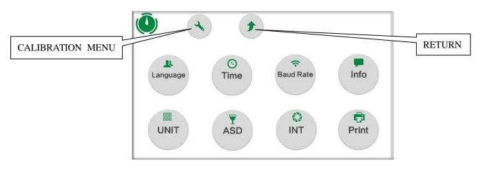
5. Press **CALIBRATION** key to enter the calibration screen.
